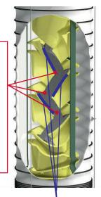
Low velocity of material in mass-flow reduces slide abrasion and minimizes dust emissions.
